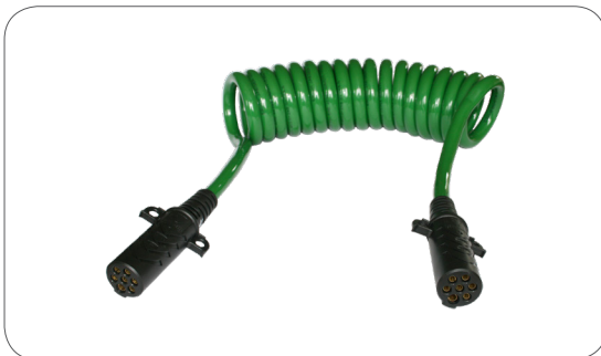
7P/12V coil - SAE J560 Primary, green cable, coil diameter: 100mm 1x 8 + 2x 10 + 4x 12 AWG (1x 8.0mm 2 + 2x 5.0mm 2 + 4x 3.0mm 2 )
