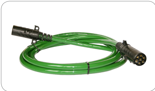
7P/12V cable - SAE J560 Primary green cable 1x 8 + 2x 10 + 4x 12 AWG (1x 8.0mm 2 + 2x 5.0mm 2 + 4x 3.0mm 2 )
